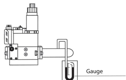
**VALVE ADJUSTMENT MULTIBLOC MB-DLE.../B01**
